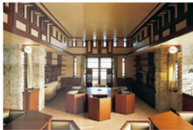
The salon of the Yamamura house includes ventilation doors in the upper part of the wall, called the clerestory. The furniture is not by Wright. YODOKO STEEL WORKS
